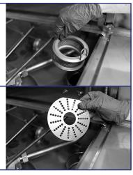
Inspect Spray Arms to ensure they rotate freely. Inspect and remove any debris in the spray jets.
