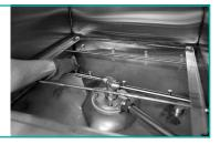
Push and hold the FILL button until the water level in the dishmachine reaches flat area of pan.
