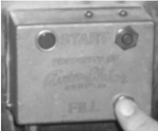
Press START button to cycle machine and dispense chemical. Verify that chemical is properly dispensed. Machine is now ready for use.
