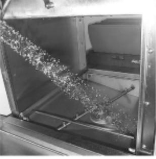
**4** Remove large debris from flat screen, if installed, located in wash tank and drain cavity.
