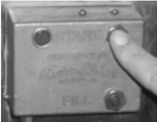
If machine is equipped with door start feature, cycle will start automatically. If not, press START button to begin cycle.
