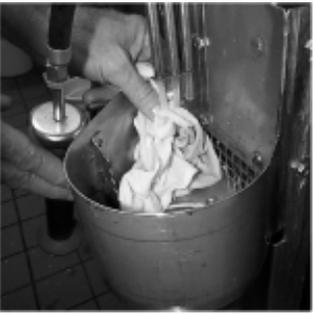
**5** Wipe interior and exterior of dishmachine with clean cloth using mild detergent solution and warm water.
